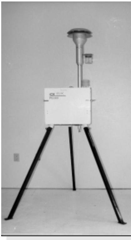
Figure 6—The BGI PQ200 Federal Reference Method PM<sub>2.5</sub> sampler.
