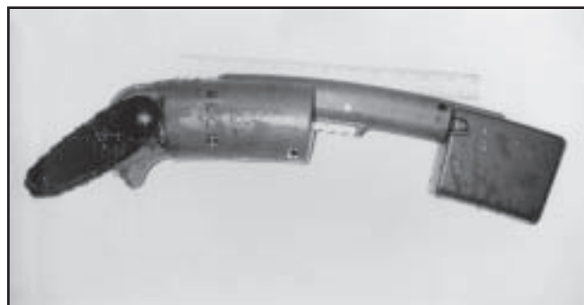
Figure 2—The Woodzig was a handy bark-scoring tool. It is no longer available.
