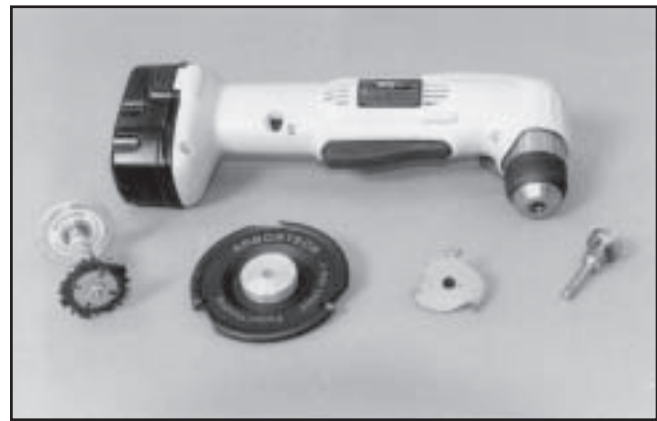
Figure 4—The DeWalt cordless right-angle drill with (left to right): Percival 2-inch carving disc, Arbortech 4-inch-diameter industrial woodcarver blade, Whiteside 2-inch-diameter, three-wing slotting cutter, and Whiteside \frac{1}{4} -inch-shank arbor with bearing.
