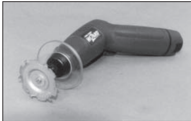
Figure 10—The Wizard cordless rotary tool with 2-inch-diameter Arbortech industrial blade and Lexan guard.
