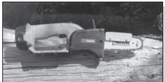
Figure 9—The MTDC modifications of the Makita cordless chain saw for bark scoring included removing the factory tip guard.
