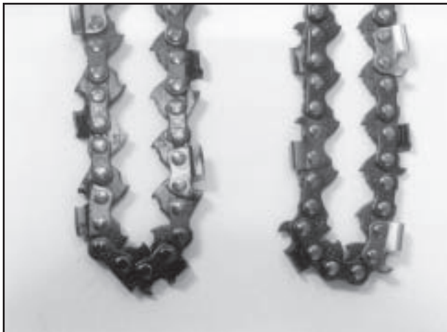
Figure 12—Cordless chain saw chains. The Makita chain on the left has two rakers for every cutter rather than one.
