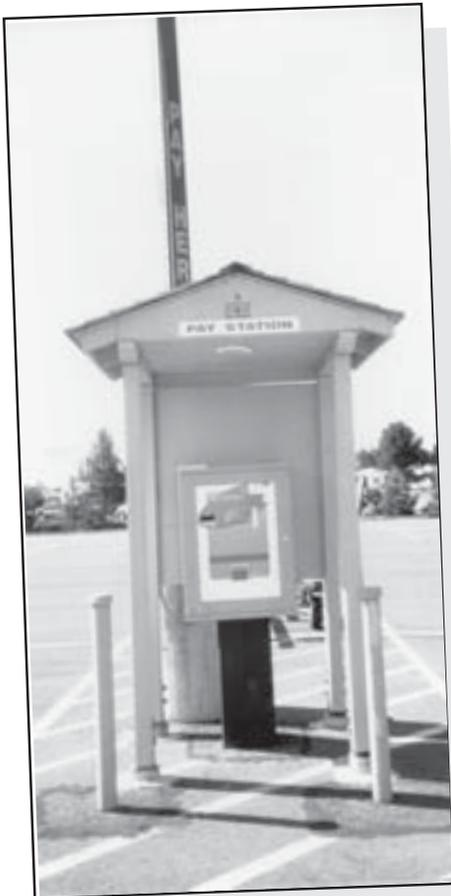
Figure 10—A tall sign allows boaters to spot the VenTek System 5 Pay Station in the parking lot even when the lot is full. Metal pipe protects the shelter and machine from vehicles.
