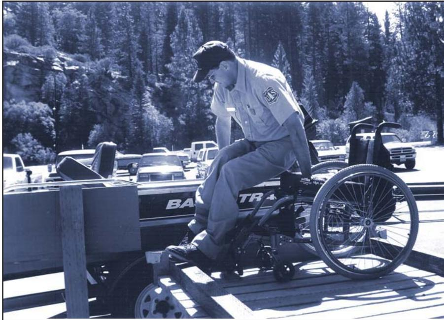
Figure 5—The boarding platform allows passengers to get into a boat while it is still on land, reducing the risks during loading and unloading.
