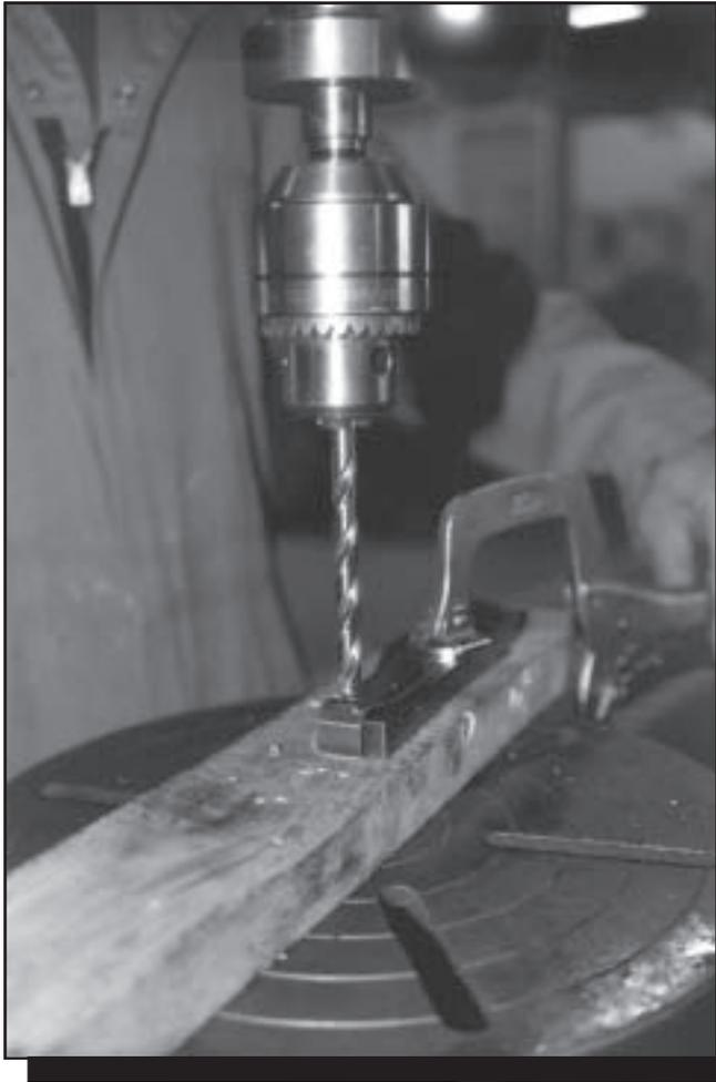
Figure 2—Drilling mounting holes in the ACCO 5 $\frac{3}{4}$ -inch banker's clip.
