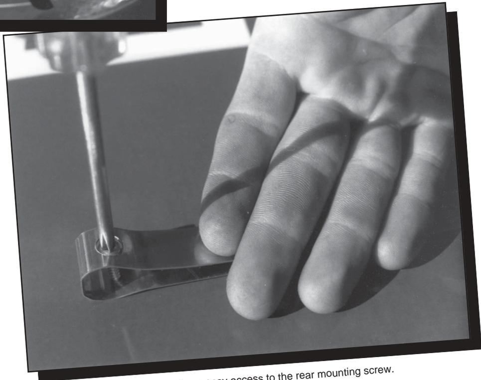
Figure 3—The large front hole allows easy access to the rear mounting screw.
