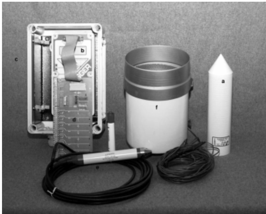
Figure 2—Equipment used for monitoring the effects of roads on groundwater piezometric surfaces. (a) PVC well tip. (b) Unidata Starlogger. (c) Weatherproof enclosure. (d) Field termination strip. (e) Hydrostatic pressure transducer. (f) Tipping bucket rain gage.
