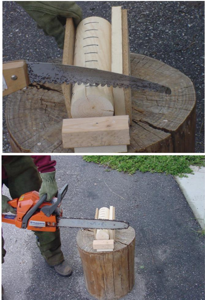
Figure 1—A jig being used with a hand saw (top) and a chain saw.
