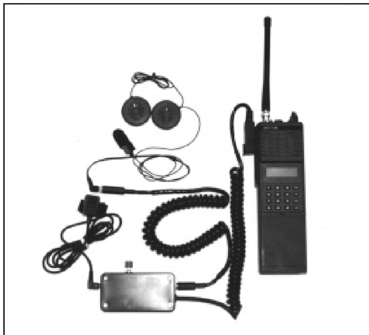
Figure 1.—Photo Of Headset Adapter And Bendix/King Radio.
