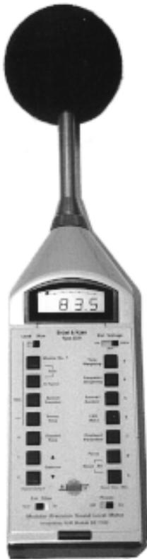
Figure 1—Sound level meter.
