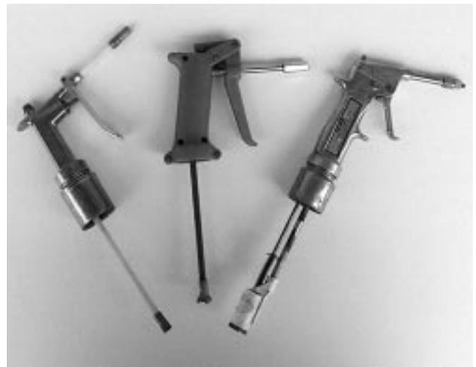
Figure 6—Three tree-marking paint guns, Panama back pack system is not shown.
