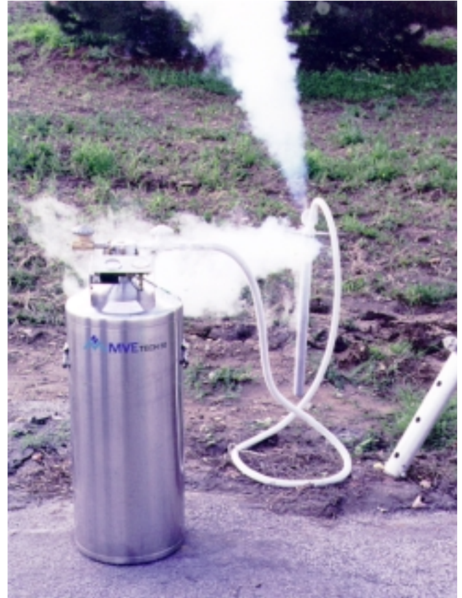
Figure 5—Liquid nitrogen released to the atmosphere as probe freezes the ground around it.
