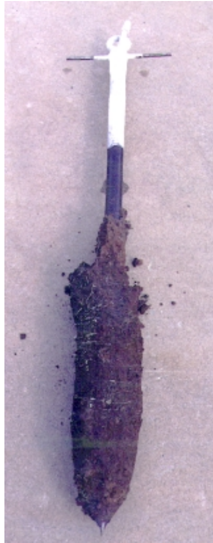
Figure 7—Sample of a frozen undisturbed core approximately 4 foot in length and 4-7 inches in diameter.
