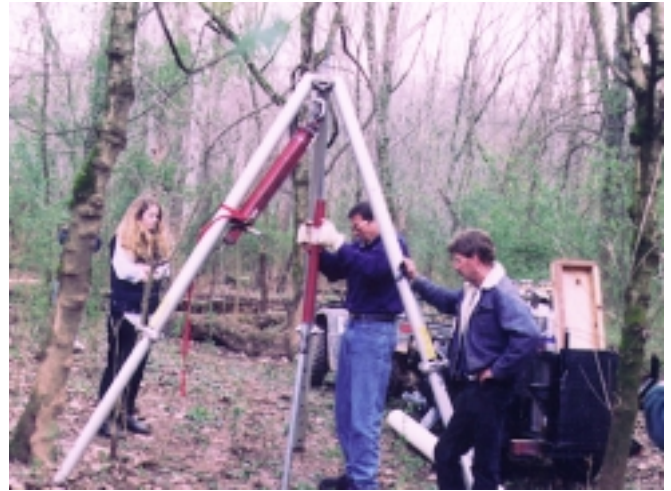
Figure 10—Skip Garrett from SDTDC pounds cryoprobe into ground using a post driver.
