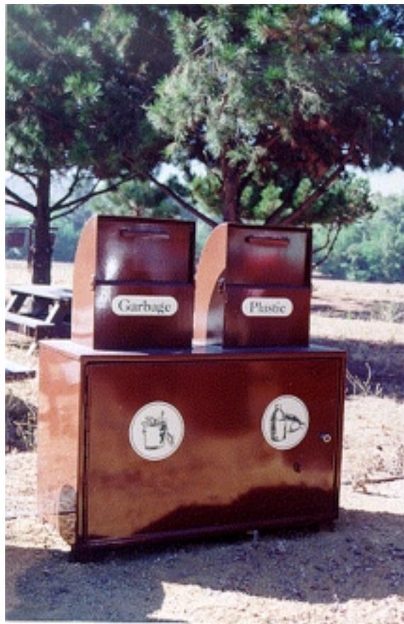
*Figure 1. Double 32 gallon bear-proof refuse container test model at SDTDC with plastic recycling option in closed position.*
