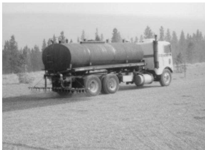
Figure 3.—Truck applying dust abatement product to landing site.
