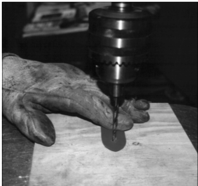
Figure 3.—Drill a hole in the strap to set pop rivet.
