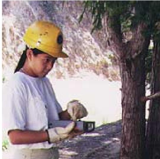
Figure 2. Power Disto rangefinder.
