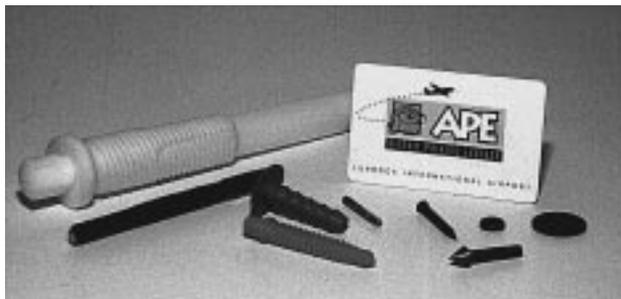
*Figure 1. Transponders are available in various sizes and shapes and have a wide range of costs and capabilities.*
