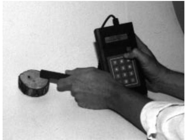
*Figure 10—Reading nail-shaped transponder (made by Microcom).*
