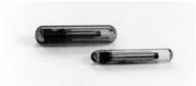
*Figure 4—Glass-encapsulated transponders are inserted into animals for identification and tracking.*
