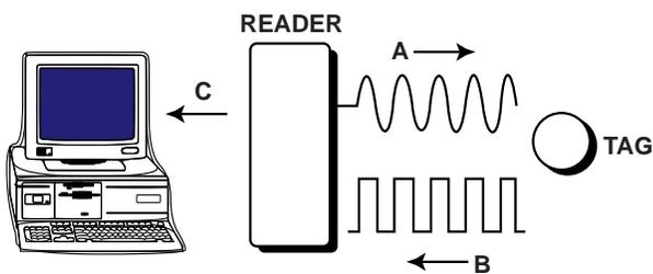
Figure 2—The reader sends a burst of energy (A) to the transponder tag. The tag responds with a coded signal (B) that is read by the reader. Data collected by the reader can be downloaded to a computer.
