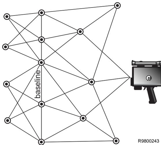
Figure 2—An example of establishing points for a site survey using a three-point resectioning technique that builds a survey from points located along a baseline.
