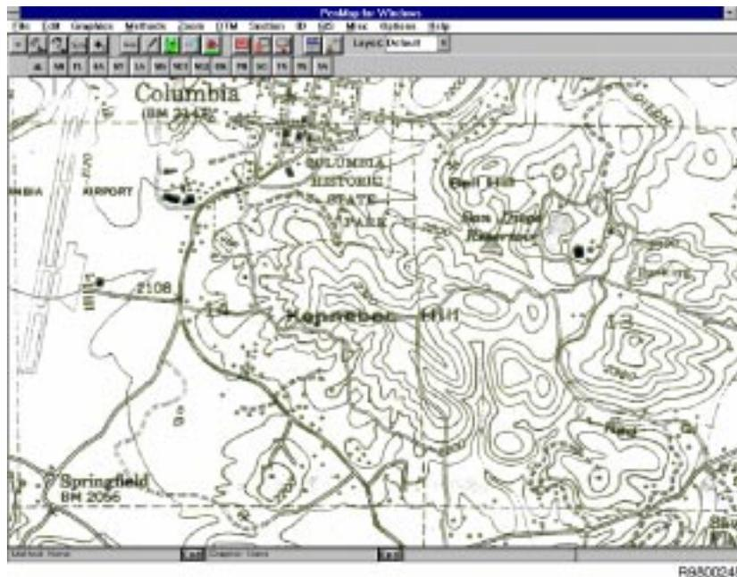
Figure 4—A raster image derived from a USGS 7.5' quadrangle is displayed in the Archsite application using Rasterback, a feature of Penmap for Windows (courtesy of Condor Earth Technologies).
