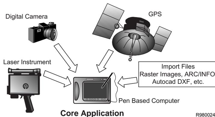
Figure 3—Various input devices of a field data-collection/mapping system.
