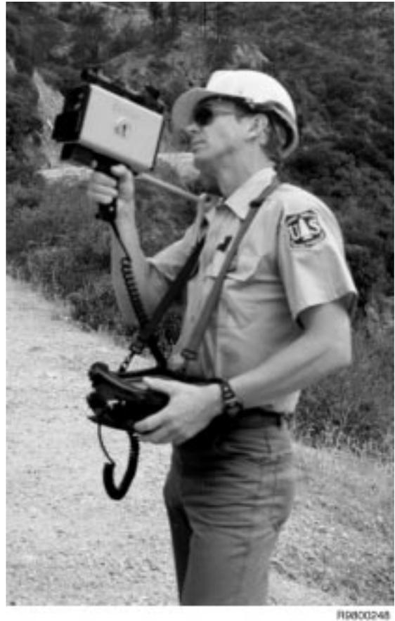
Figure 7—Operator with pen-based computer receiving input from a Laser Technology, Inc., Criterion 400 laser survey instrument. Computer is a ALPS, Inc. Kalidor 2500 pen-based computer (no longer manufactured).
