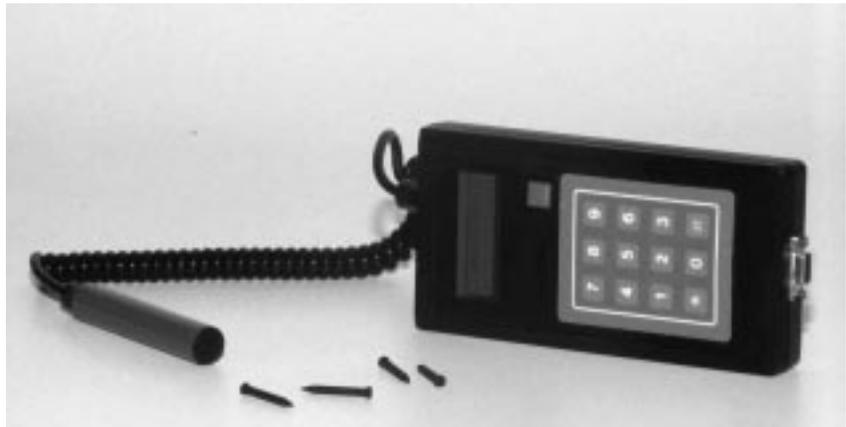
*Figure 3. Nail-shaped transponders with reader (made by Microcom).*
