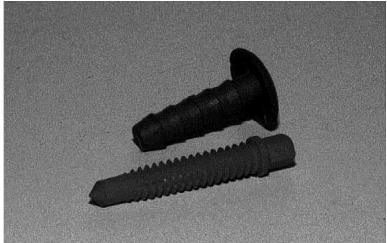
*Figure 2. The screw-in shape (made by Rydex) and the press-in shape (made by EID) were tested on the Tongass NF.*
