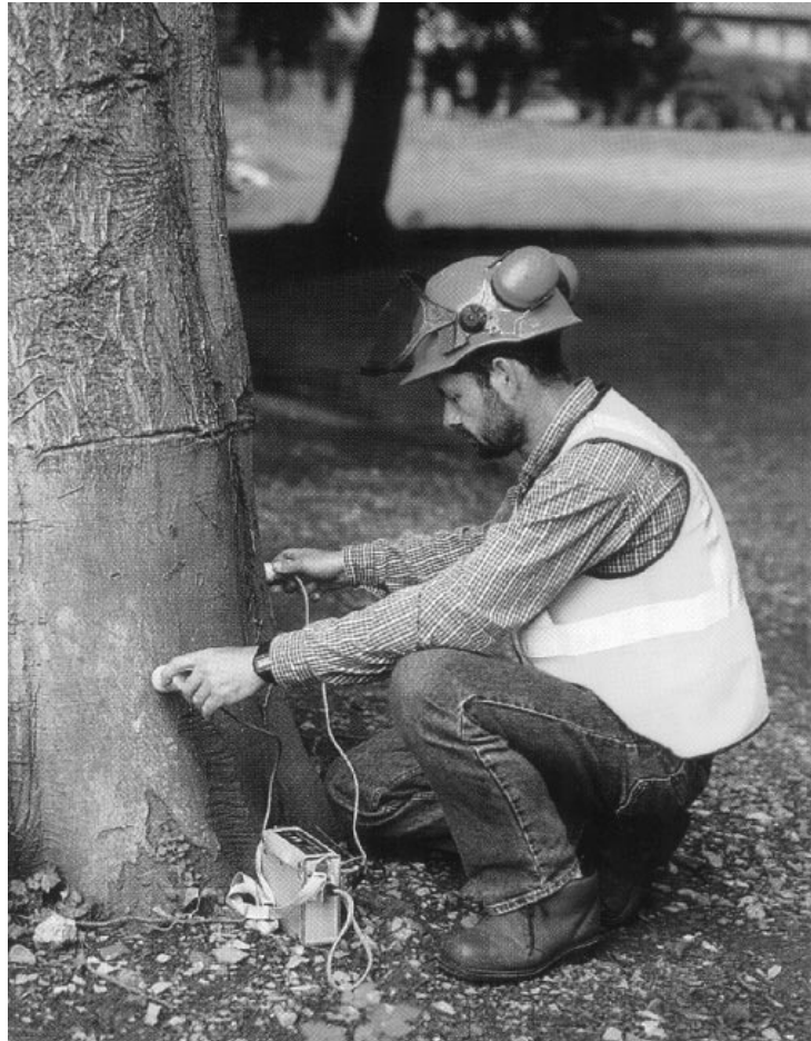
Figure 6. Arborsonic Decay Detector.
