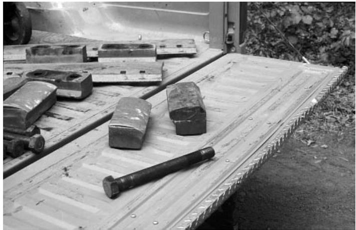
Figure 6. Attachment bolts and worn hammers.
