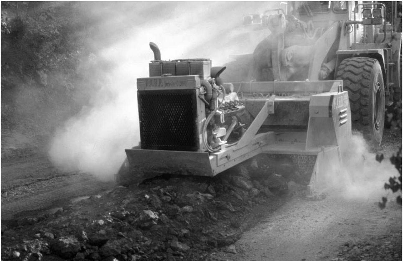
*Figure 8. Forester C-2000 grinding through windrow.*
