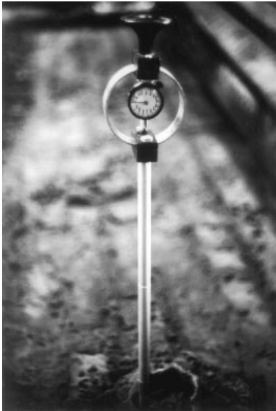
Figure 5. Cone penetrometer device.
