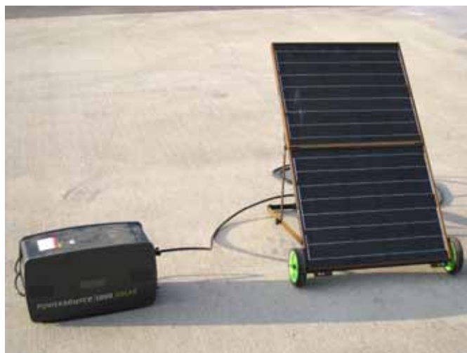
Figure 7. Ecotricity 1800 solar generator with solar panel.
