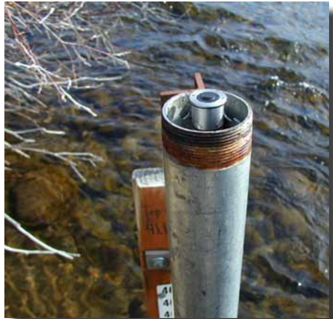
Figure 13. Top of Ott "Mini" in pipe, located to allow download.
