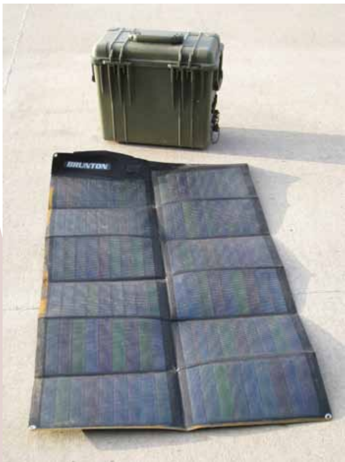
Figure 8. MTDC power unit with folding solar panel.
