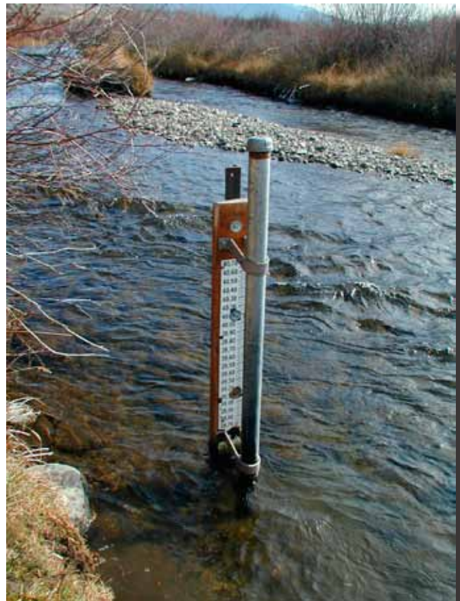
Figure 11. Typical stream gauge.
