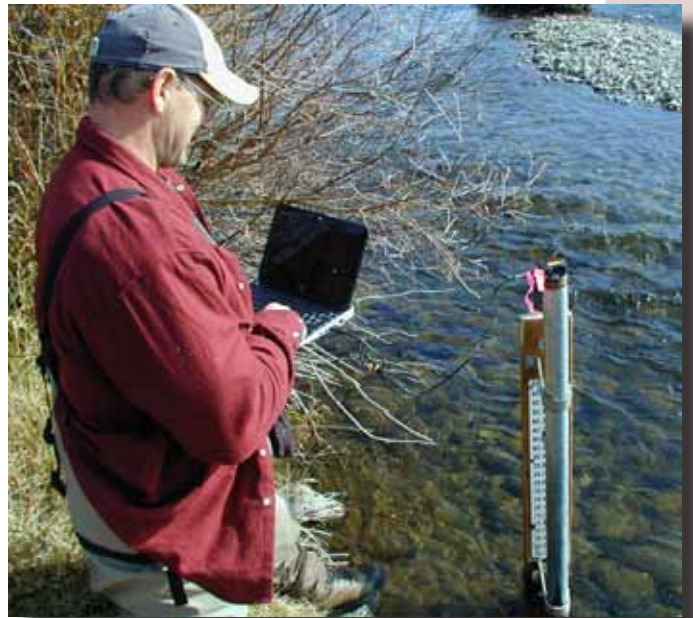
Figure 14. Downloading using optical reader
