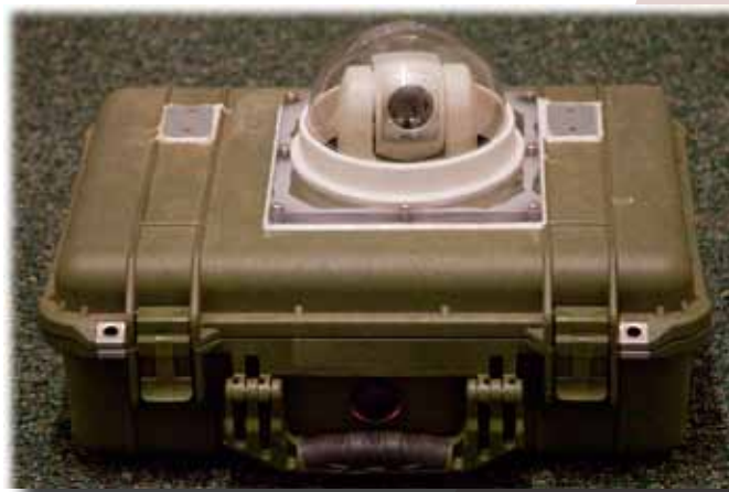
Figure 3. Photo of a weatherproof HD pan, tilt, and zoom camera that operates on cellular networks.
