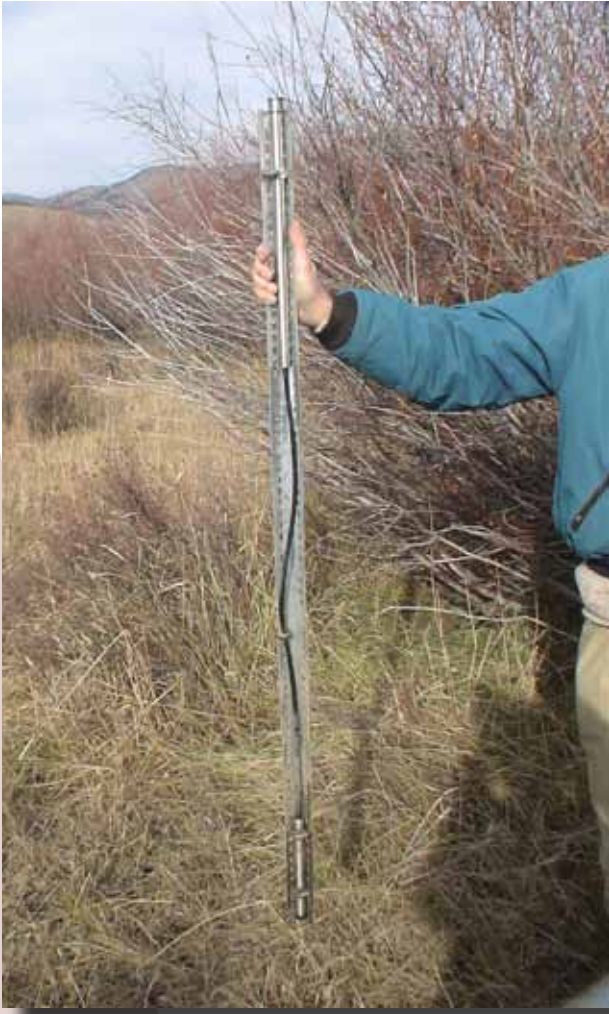
Figure 12. Ott "Mini" attached to sleeve that slides in pipe.
