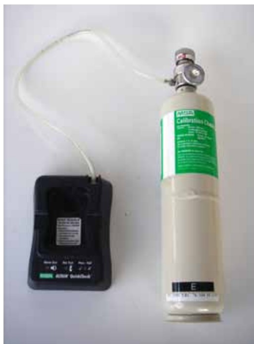
Figure 1—QuickCheck Station with calibration gas.
