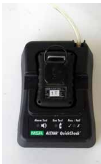
Figure 2—QuickCheck Station with dosimeter.
