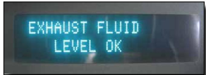
Figure 2—Normal diesel exhaust fluid status displayed on vehicle message center (2011 Ford F-450).
