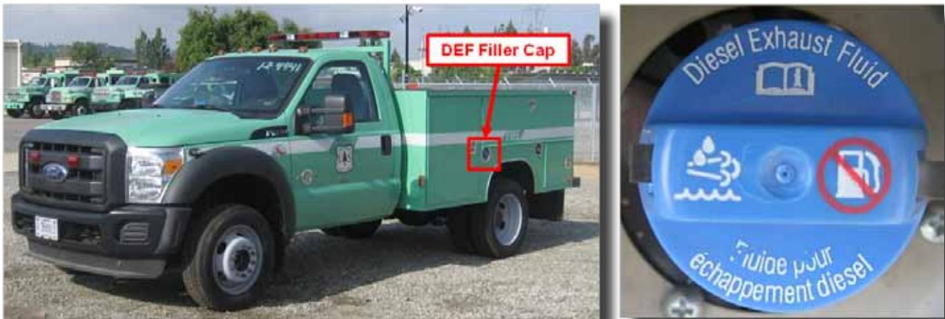
Figure 1—Diesel exhaust fluid filler cap located on 2011 Ford F-450 with utility body (selective catalytic reduction systems only).
