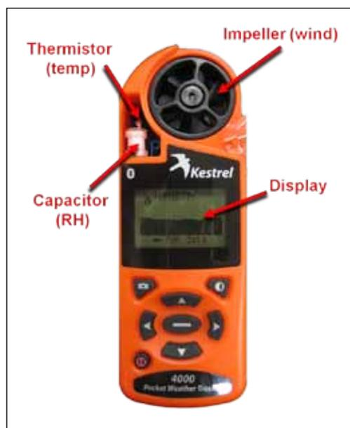
Figure 3—Nielsen Kellerman Kestrel 4000 electronic weather meter.
