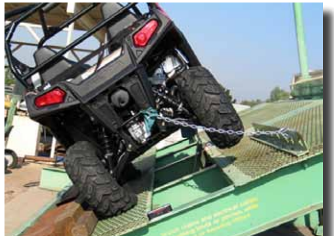
Figure A20—The RZR rolls at 32.9 degrees.
