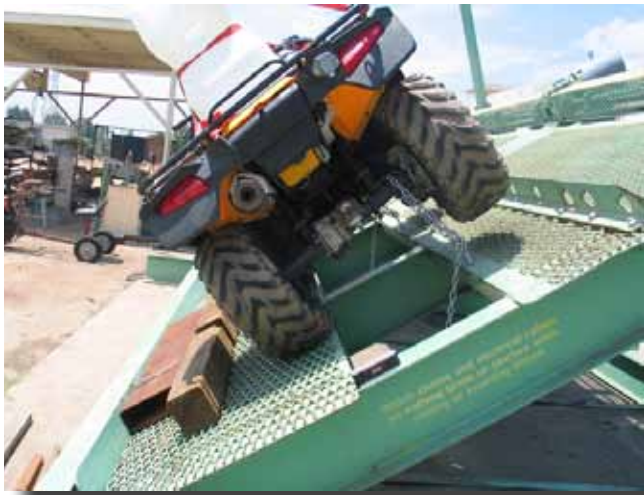
Figure A12—Rubicon ATV rolls at 34 degrees.
