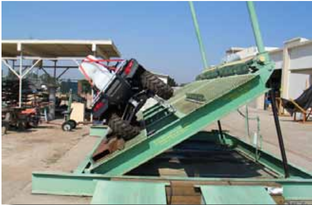
Figure A16—The Rincon rolls at 32.2 degrees.
