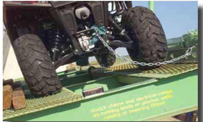
Figure A19—Front tire of the RZR is off the table at 30.8 degrees.
