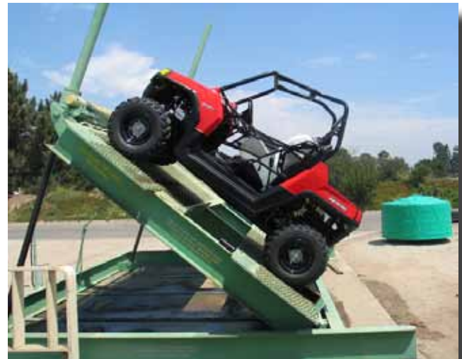
Figure A23—RZR at 40 degrees. Security ropes are still slack and RZR is on blocks.
