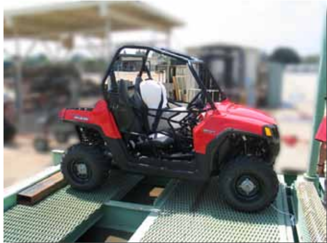
Figure A22—The RZR ready to begin the longitudinal test.
