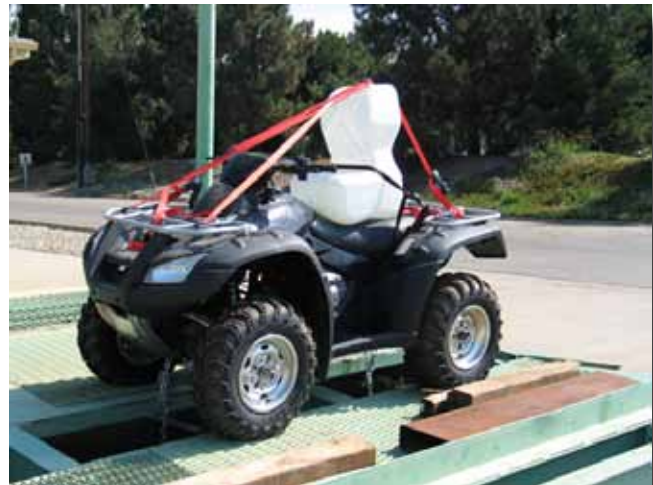
Figure A3—Rincon chained to the table for the lateral test.
