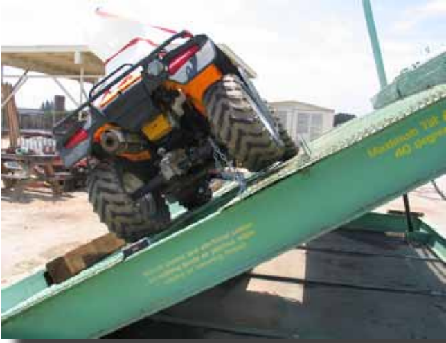
Figure A11—The Rubicon's rear wheel lifted at 27.5 degrees.
