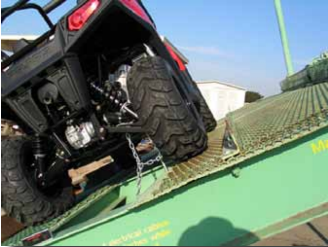
Figure A21—The right front tire lifted off at 30.8 degrees.
