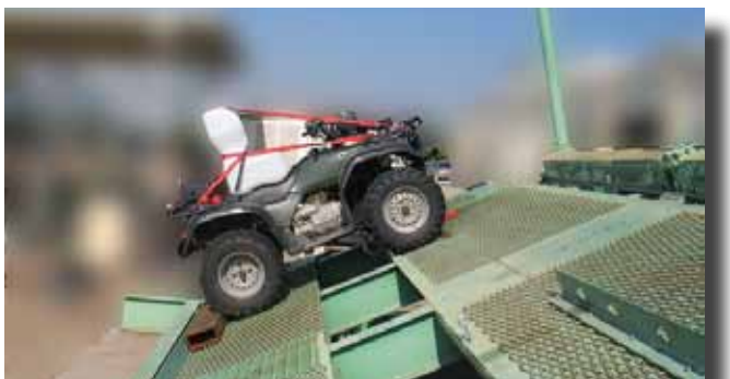
Figure A10—Because of the brakes releasing and catching, the Foreman ES's rear tires at the end of the test are on the blocks at 40 degrees.
