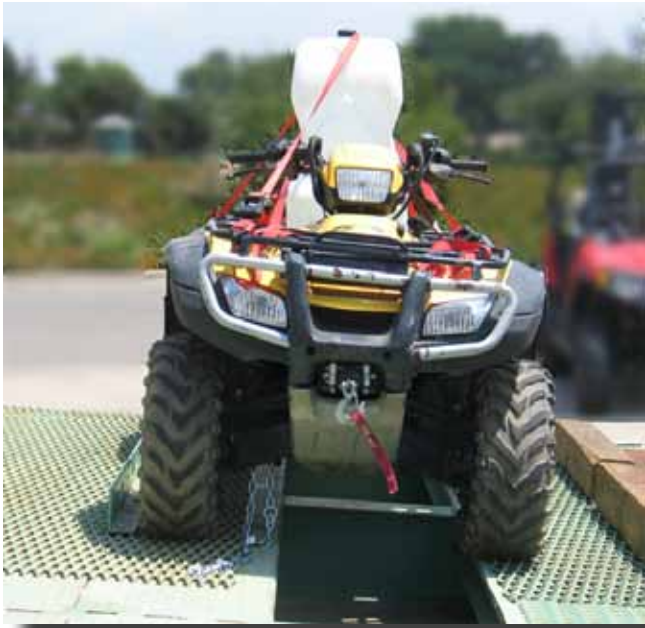
Figure A1—Foreman ES strapped and ready for the lateral test. There is a winch and a fire extinguisher on the front and a trailer hitch on the back that add weight.
