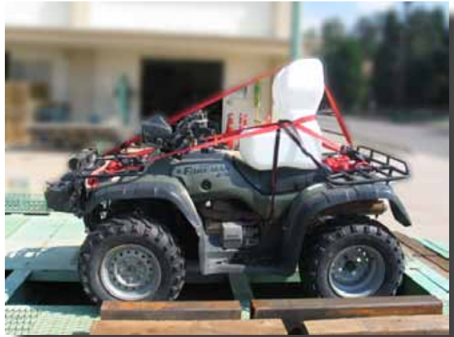
Figure A2—The Rubicon shown strapped during the lateral test. There is a winch on the front and a trailer hitch on the back that add weight.
