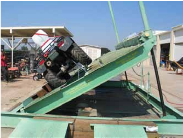
Figure 1—Tilt table shown at 40 degrees.
