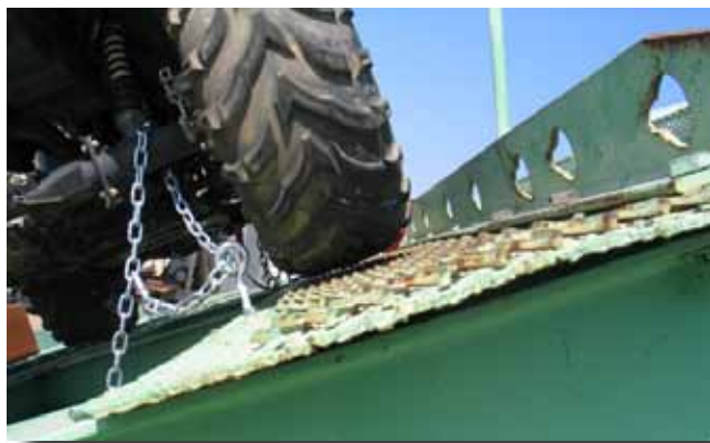
Figure A7—Foreman ES rear wheel lifted at 27.4 degrees.
