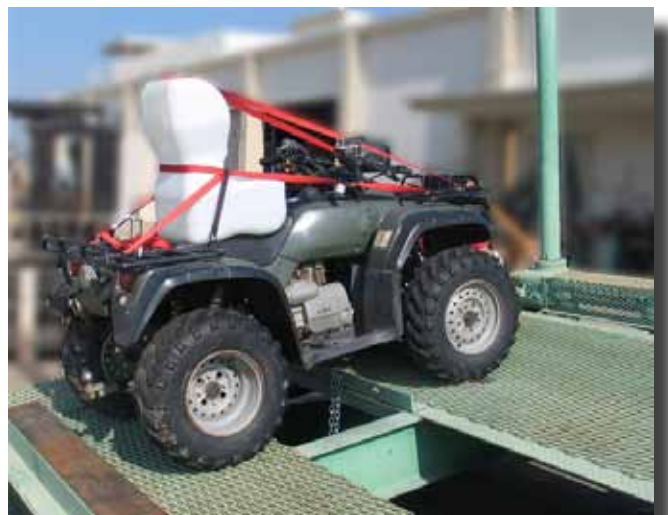
Figure A9—The Foreman ES beginning the longitudinal test. Notice that the rear tires are several inches from the blocks.
