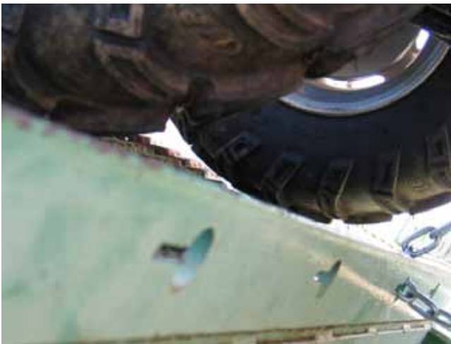
Figure A17—The right front tire lifted off at 39.5 degrees.
