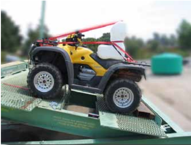
Figure A5—Dummy strapped for longitudinal test. Note the strap around the “neck” to keep the dummy from tilting backwards.
