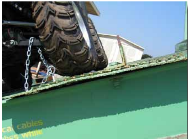
Figure A14—The Rincon front tire, in right portion of photograph, is barely off the table at 30.0 degrees.
