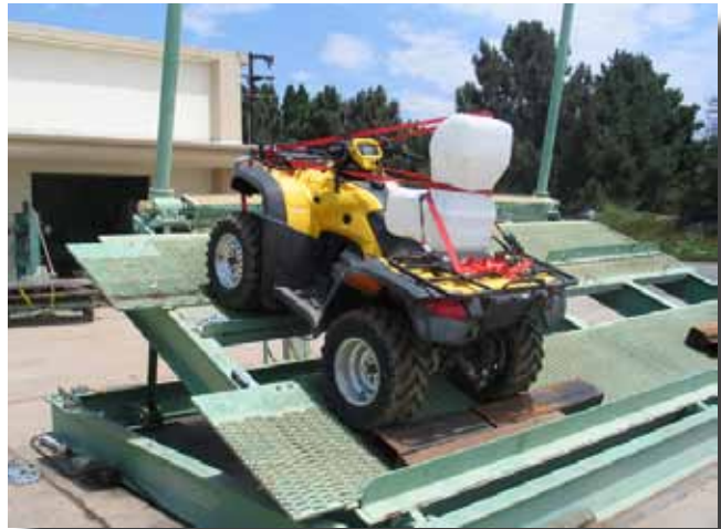
Figure A13—The Rubicon's rear tires on blocks at 19 degrees.
