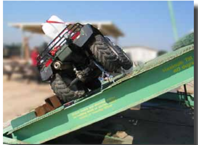
Figure A8—Foreman ES at rolling point, 30.9 degrees.
