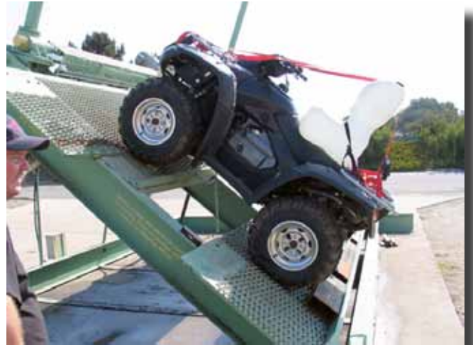
Figure A18—The Rincon tilted at 40 degrees.
