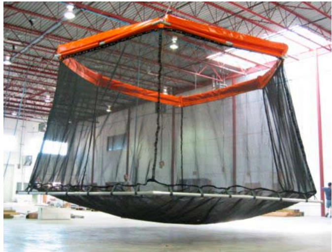
Figure 3. View of fish strainer suspended in air.
