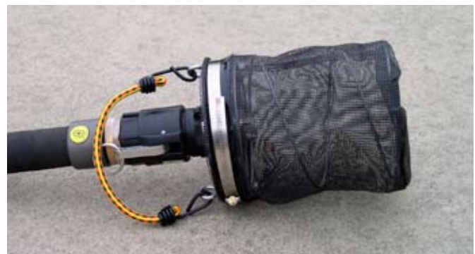
Figure 2. Hose-end fish strainer for drafting operations.
