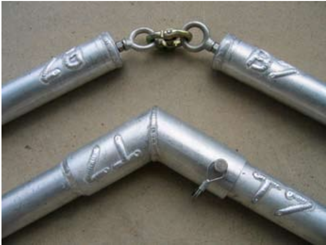
Figure 4. Corner pieces include labels for ease of assembly.
