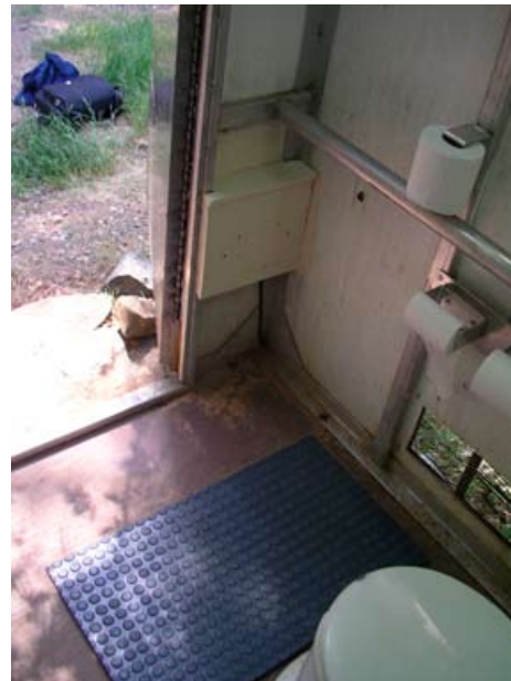
Figure 2. Pressure-mat counter installed in toilet.
