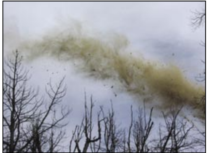
Figure 8—Dispersion of straw dropped from 150 feet at 50 knots.
