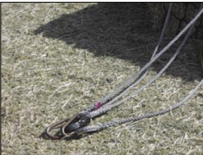
Figure 4—Rodeo method, net ready for hook up. The retrieval line attaches to cage of remote hook and rings on net attach directly into remote hook.
