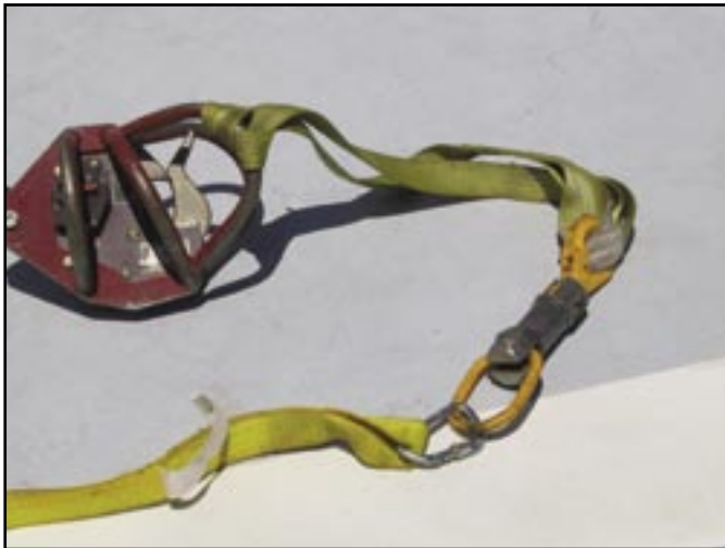
Figure 2—Rodeo method, showing attachment of retrieval lines to remote hook.
