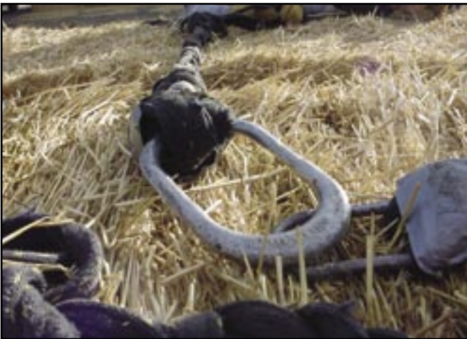
Figure 7—Preferred steel rings for Brownell nets.
