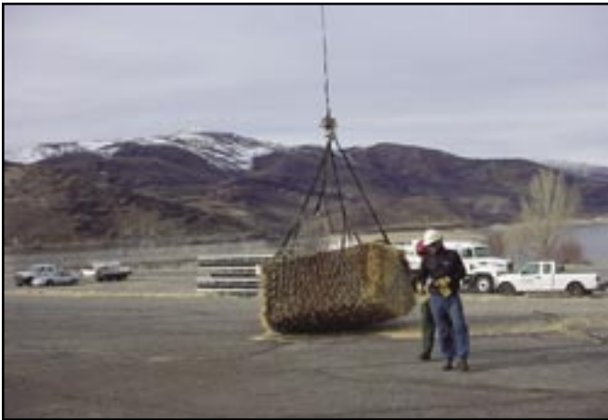
Figure 5—Biscuit method, one steel ring is attached to the cage of the remote hook. The other three rings are attached directly into the remote hook.
