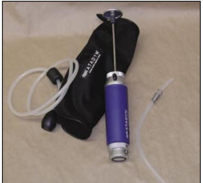
Figure 11—The Pocket Filter has a plunger-type pump.
