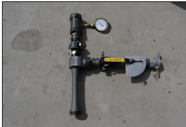
Figure 1—T&D-developed retardant mixer for SEAT bases.
