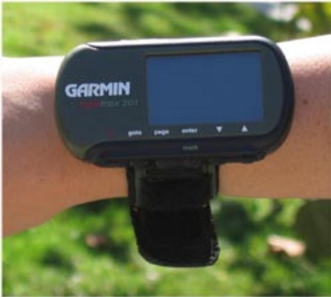
Through testing it was determined that the Foretrex could be placed inside the firefighters web gear and still obtain a good GPS fix. This placement helps protect the unit and also eliminates the need to have the device on the firefighter's wrist, where it could be exposed to damage or interfere with the firefighter's work. Placing this device on the crewmembers, provided a daily log of the firefighters movement. This data can then be used to supplement the GPS data acquired with the GeoXT.
