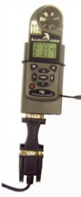
The Kestrel 4000 Pocket Weather Tracker is a handheld weather meter that measures, records, and displays the following readings:
