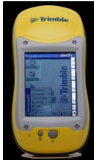
The GeoXT offers the functionality of a personal computer, containing programs such as Pocket Word and Pocket Excel. Windows Mobile 2003/5 also allows the user to install third party software or customized software to aid in collecting data.
