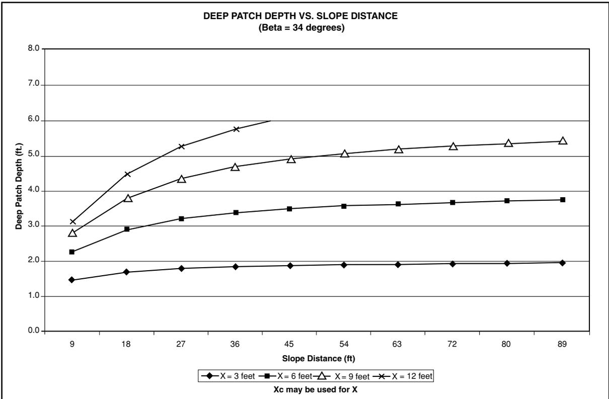
Figure 6—Deep patch vs. slope distance.
