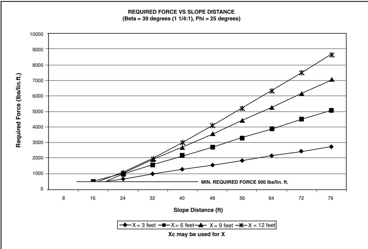
Figure 11—Required force vs. slope distance.
