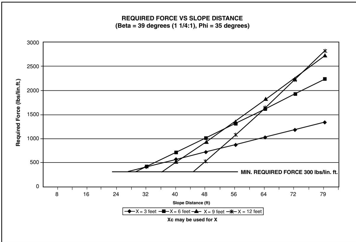
Figure 13—Required force vs. slope distance.
