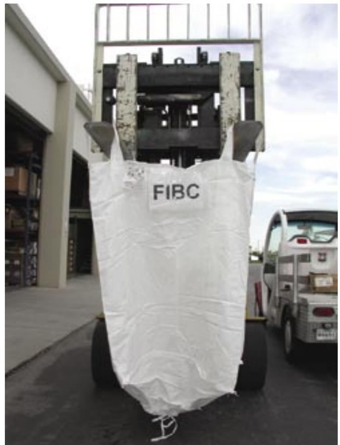
Figure 1—FIBC carried by a forklift.
