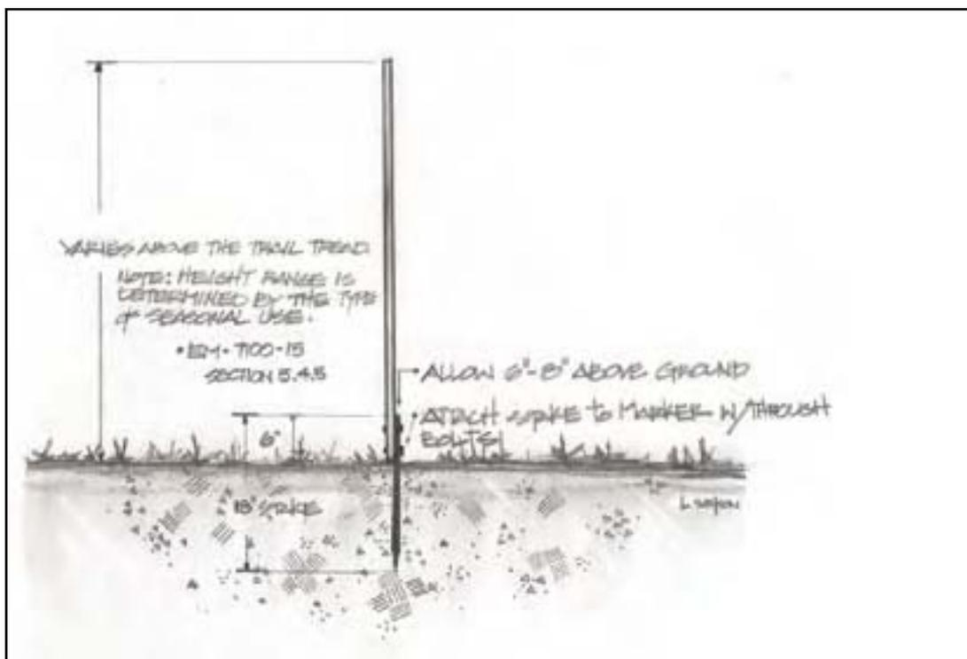
Figure 26—Schematic of trail marker installation.
