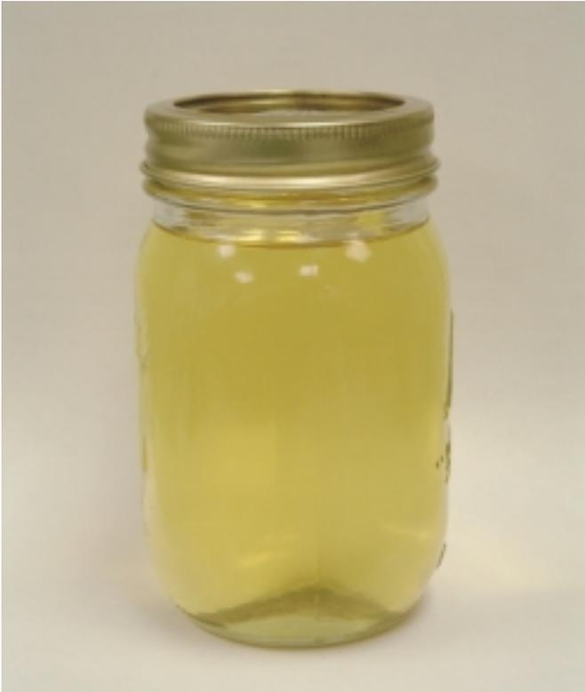
Figure 1 Pure biodiesel fuel (B100) made from recycled cooking oil.
