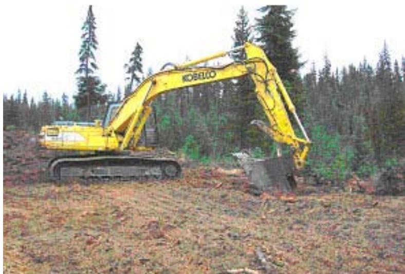
*Figure 6b. Subsoiling using the SEB.*
