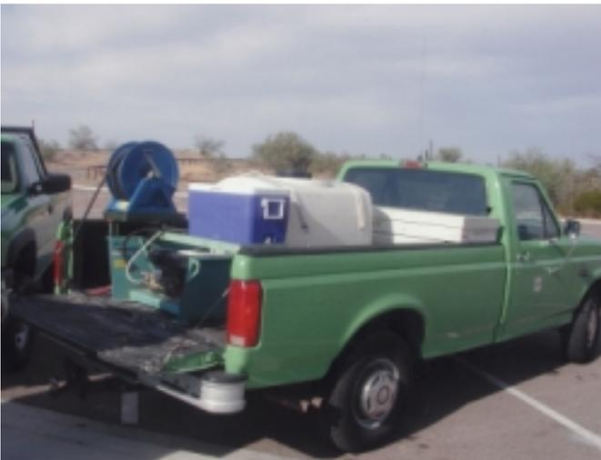
Figure 3—Marsh Industries skid mounted slip-on pressure washer.
