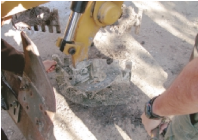
Figure 4—Rotating blade to adjust angle.
