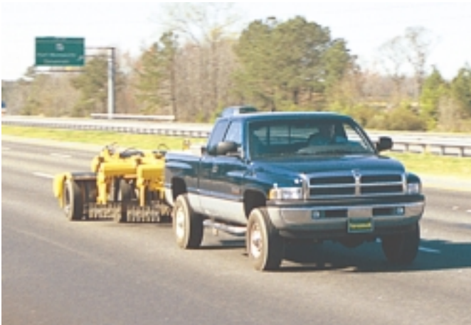
Figure 13—Grader pulled by a heavy-duty truck.
