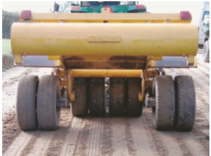
Figure 6—Compacting tires and weight.
