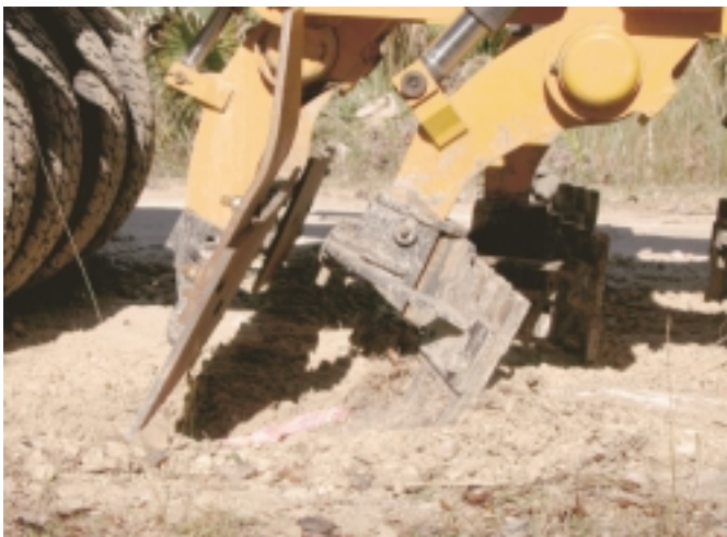
Figure 9—Blade hydraulic system absorbing the impact of boulder.
