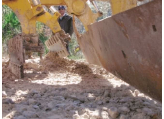
Figure 10—Notice how offcenter the blade is when taking the impact.
