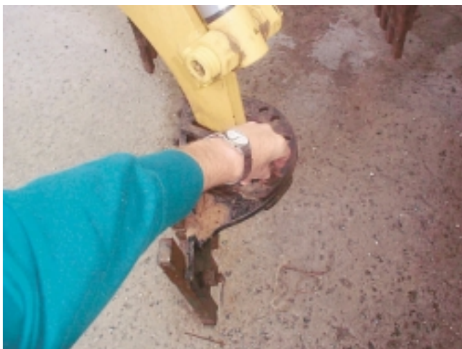
Figure 5—Pulling pin to adjust angle.
