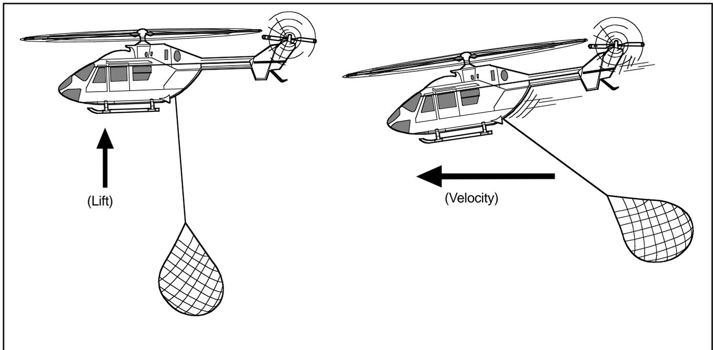
Figure 5—Force caused by snagging load.
