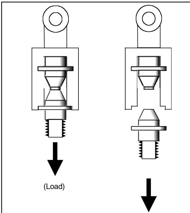
Figure 3—Tensile design.
