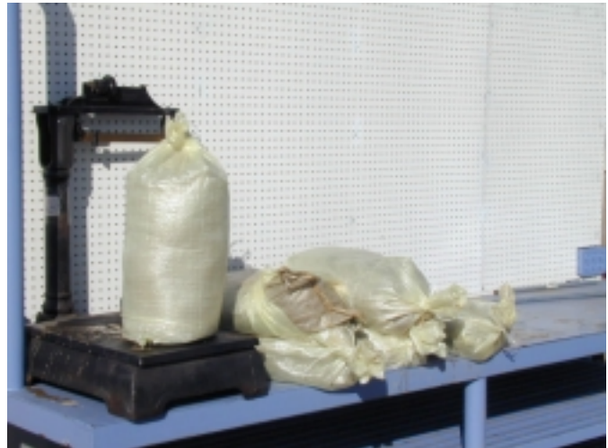
Figure 3—Double-bag for increased strength.
