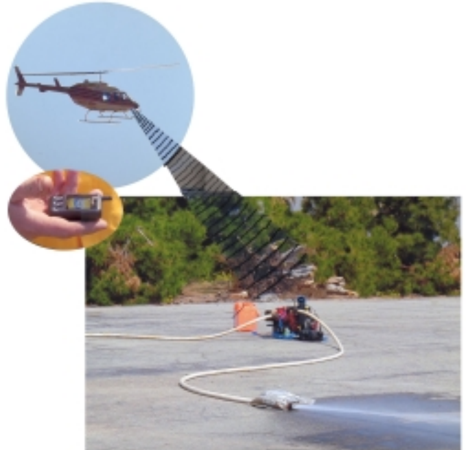
Figure 7—Testing remote pump system from a helicopter.
