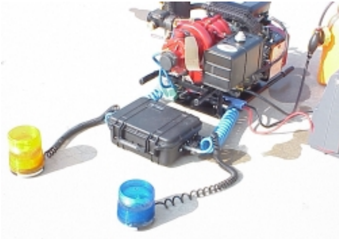
Figure 5—Lights flash to indicate pump is operating.
