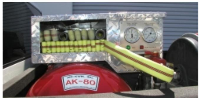
Figure 1—The Air-Kwik unit comes with a 50-, 80-, or 100-gallon size water tank and includes a hose tray compartment.
