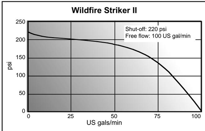
Figure A18–Striker II pump performance curve.
