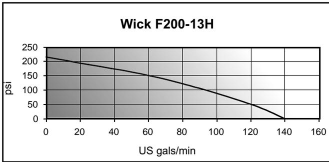
Figure A22–Wick F200-13H pump performance curve.
