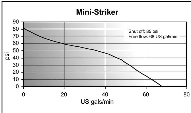
Figure A11–Mini-Striker pump performance curve.
