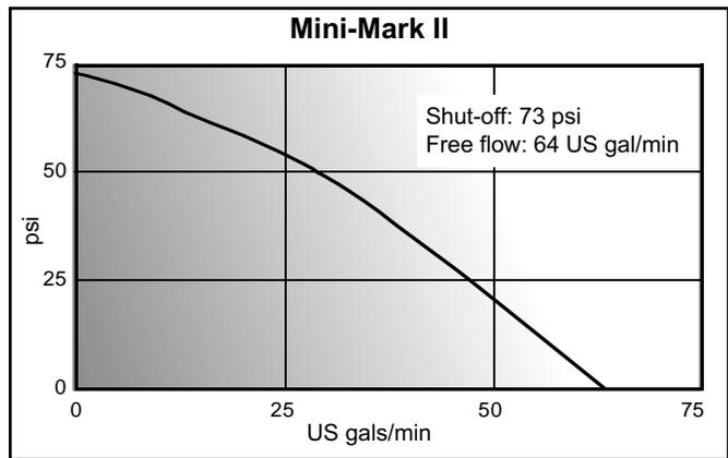
Figure A5—Mini-Mark II pump performance curve.
