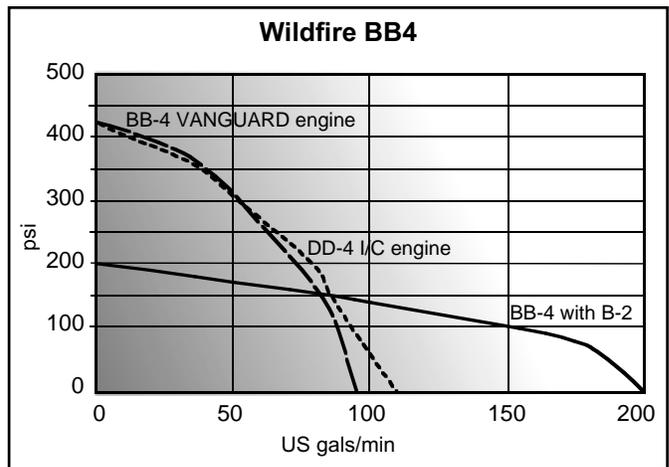
Figure A28–BB4 pump performance curve.
