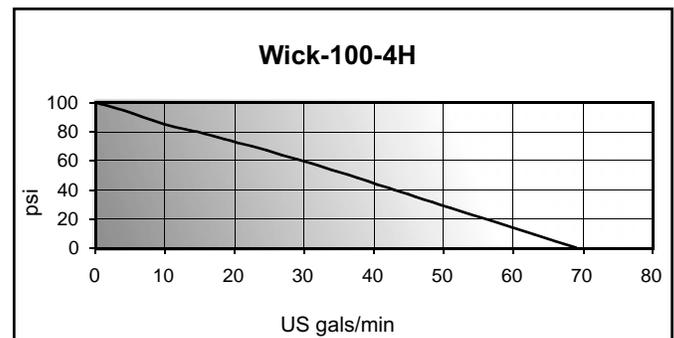
Figure A9–Wick-100-4H pump performance curve.
