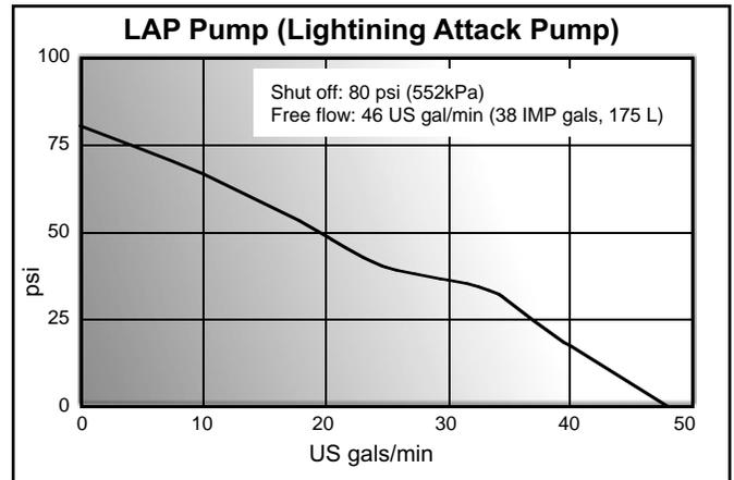
Figure A2-LAP pump performance curve.
