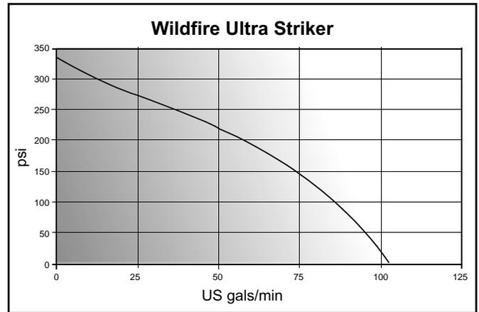
Figure A24–Ultra-Striker pump performance curve
