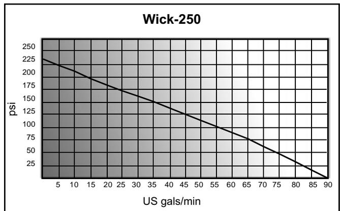
Figure A13–Wick-250 pump performance curve.
