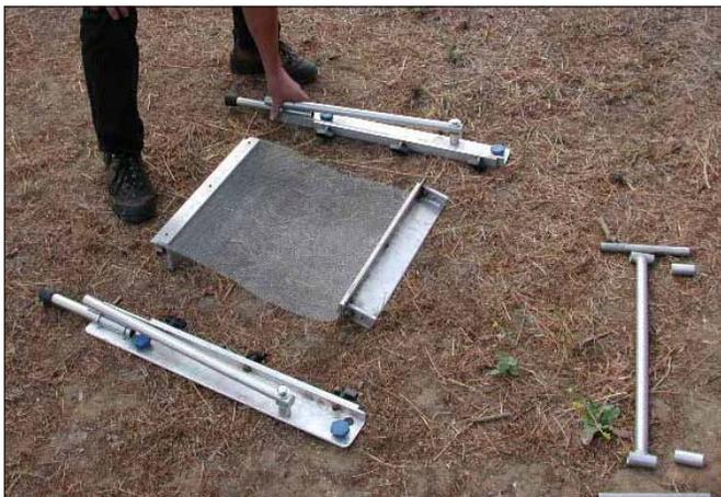
Figure 4—The side member subassemblies are placed beside the screen.
