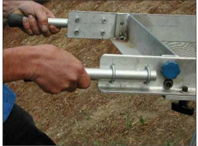
Figure 9—Screen box handles are 10-inches long.
