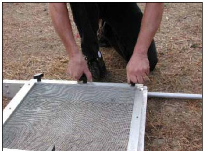
Figure 6—The Tee nuts are placed over the studs and tightened firmly.
