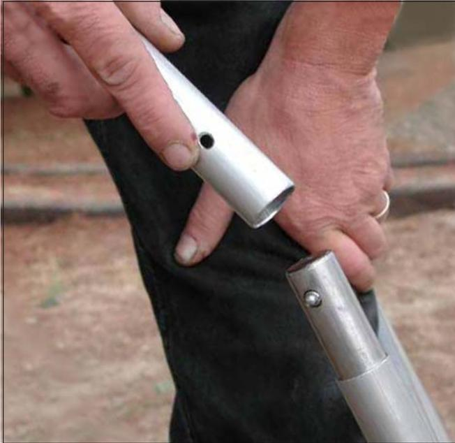
Figure 11—The plungers snap into their respective positioning holes.
