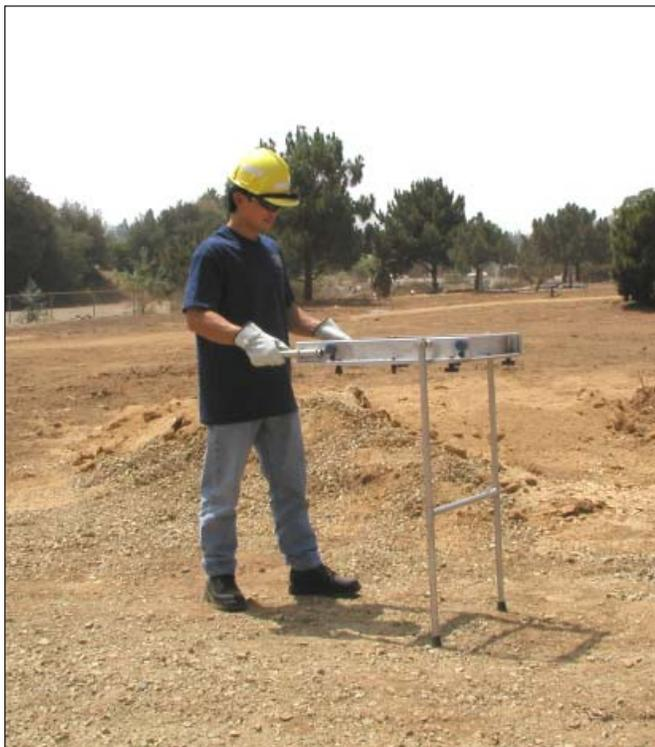
Figure 1—Collapsible aluminum archeology screen.
