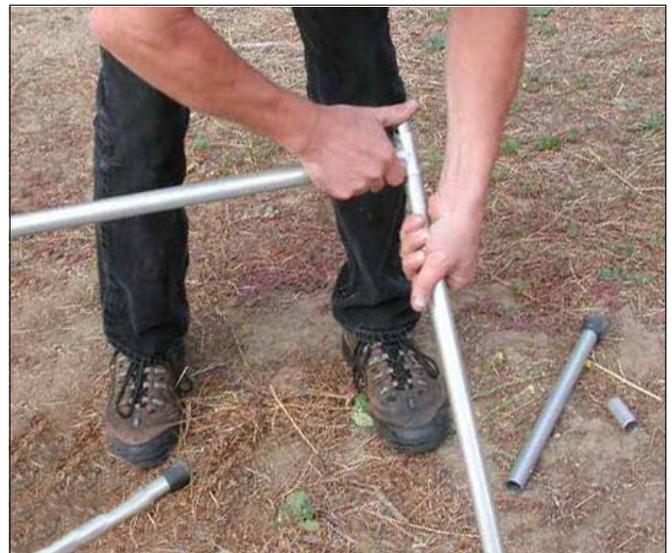
Figure 10—The crossmember slides over the connector and the other side of the crossmember aligns with the opposite leg.
