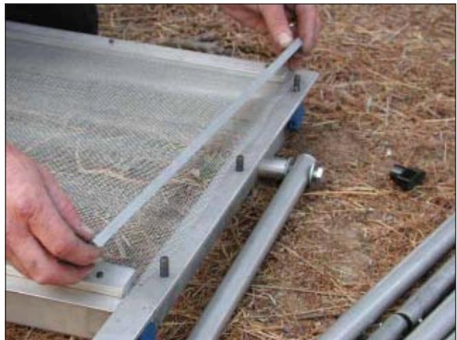
Figure 5—The screen clamp strip is placed over the three studs.
