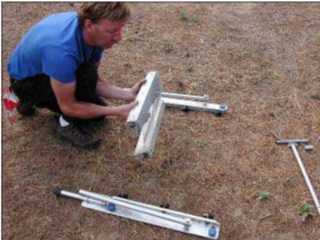
Figure 3—The screen that is attached to the lateral subassembly is unrolled.
