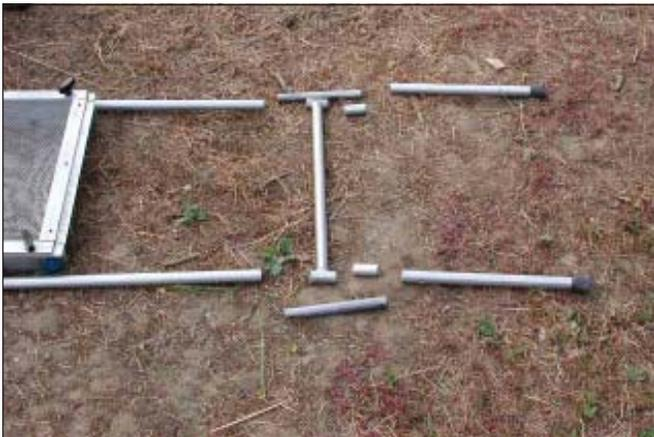
Figure 8—Spacers may be positioned above or below the crossmember.
