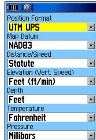
**Situations Where Position Format And Map Datum Are Critical** - A Garmin receiver's **Position Format** and **Map Datum** settings aren't typically a critical issue if users upload or download tracks and waypoints electronically using DNRGarmin or MxGPS, for instance. Remember, **Position Format** and **Map Datum** settings only affect on-screen coordinate display, not internal data capture and storage.
