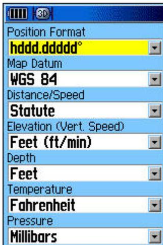
**Position Format And Map Datum** - Garmin GPS receivers capture and store positions as decimal degrees of latitude and longitude referenced to the WGS84 datum. Although users can set how GPS positions are displayed on-screen, those settings have no effect on how the GPS positions are actually captured, or stored, internally.
