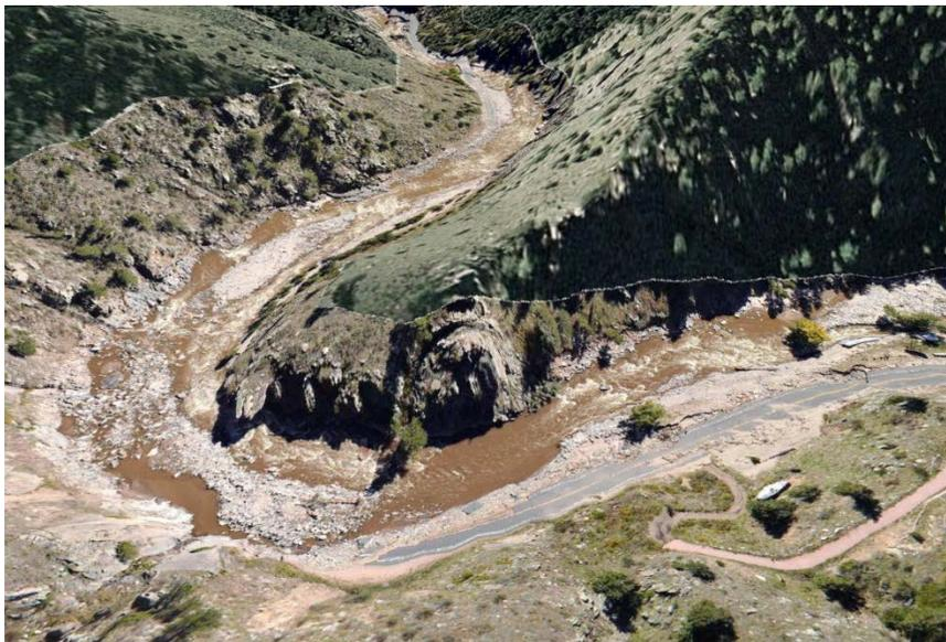
**Figure 1:** Eradicated US-34 roadway embankment along the Big Thompson River on the Roosevelt National Forest (10/21/2013). Peak discharge =  $\sim 430 \text{ m}^3/\text{s}$  (15,000 cfs);  $\omega = 2700 \text{ W/m}^2$ . Flow direction is away from viewer. Graphic created in ArcGlobe with imagery from the Colorado Department of Transportation and LiDAR data from FEMA and USGS.
