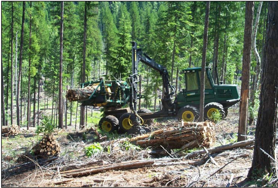
Figure 2. The Timberjack 1490D Slash Bundler.
