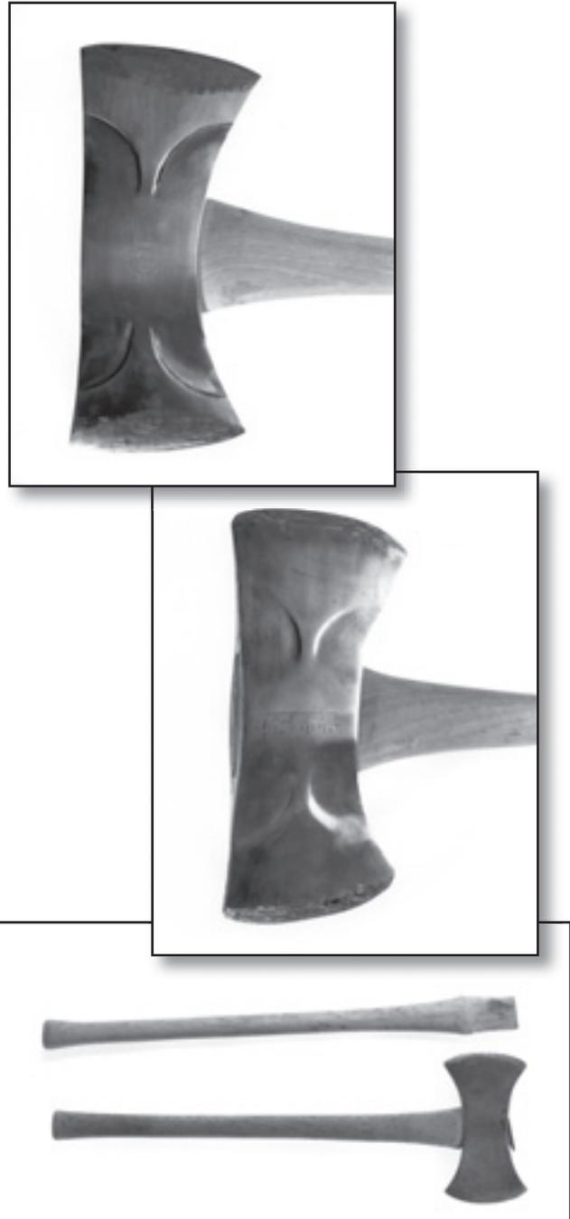
Figure 15—Three representative double-bit patterns: Bluegrass Western pattern double-bit ax (top); True Temper Kelly Perfect Michigan pattern double-bit ax (middle); and a 2<sup>1/2</sup>-pound reversible cruiser ax, sometimes used for ax throwing (bottom).
